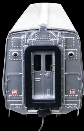
Factory-installed, separate diaphragms and grab irons
